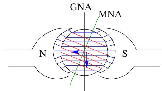
Figure 1: Armature reaction
