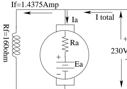
Figure 2: DC shunt motor
