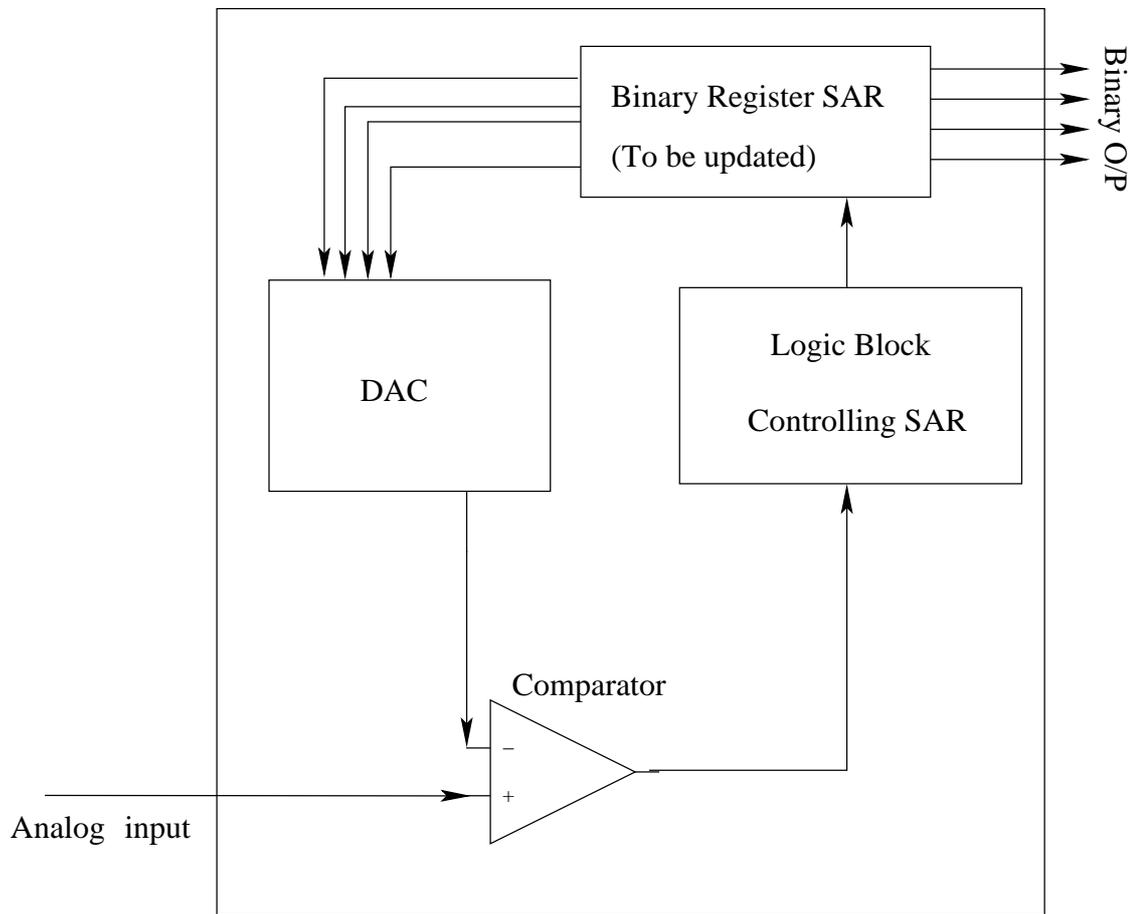
Figure 2: ADC block diagram
