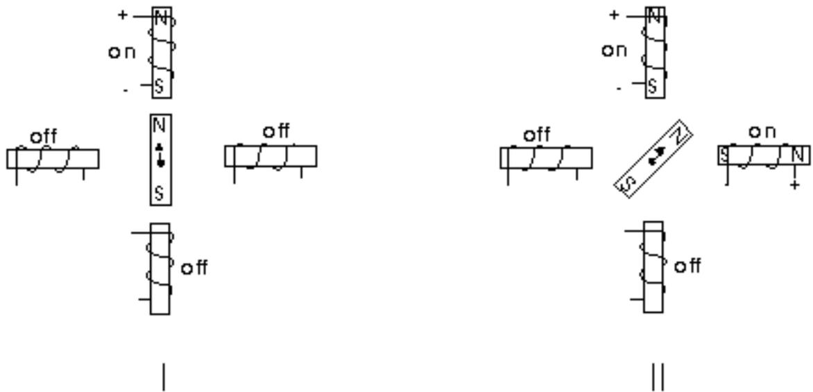
Figure 2: Half stepping of stepper motors
