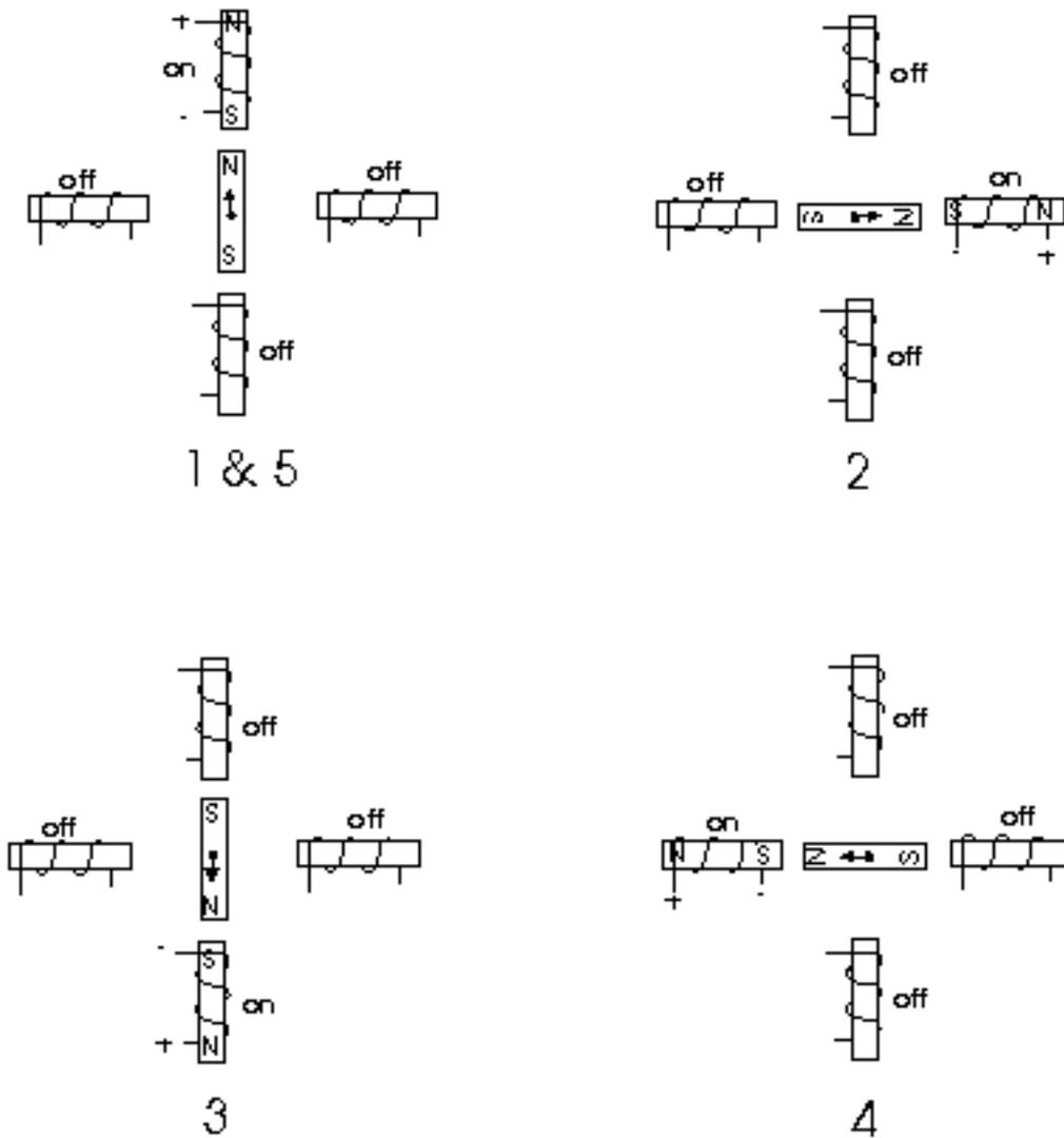
Figure 1: principle of stepper motor
